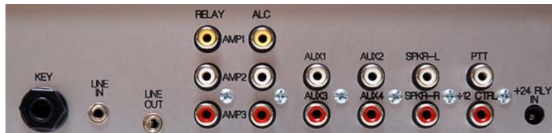
The rear panel circuit board attaches to the rear panel with six No. 4 x 3/8" sheet metal screws and the nuts on the jacks.
