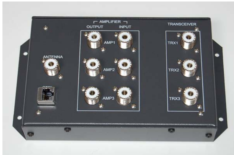
The completed StationPro RF relay unit
