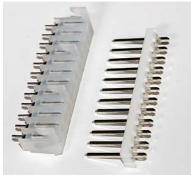
12 pin Molex 0.156” female PCB connector and matching 12 pin header
