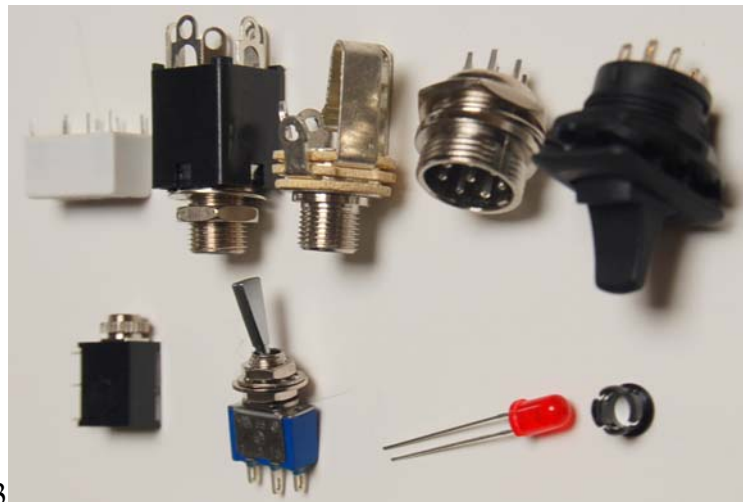
Principal SP-I Front Panel Components. Top row (left to right): K301, J302, J301, mic jack, S301. Bottom row: J303, S302-S305, LED, Led bezel
