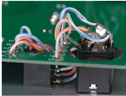
Detail showing wires from jacks threaded through the access holes on the front panel printed circuit board. Be sure none of the wires interferes with the jacks' operation
