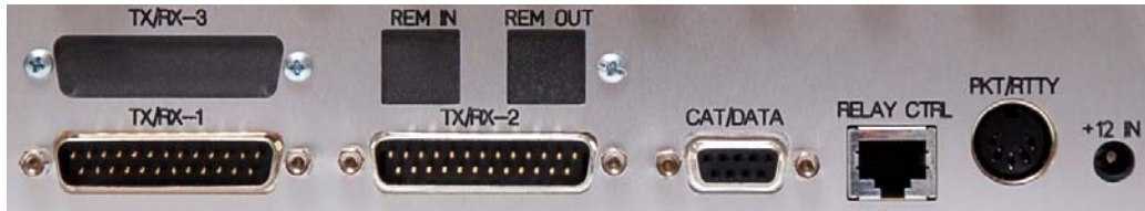
The main circuit board attaches to the rear panel with six jack screws. Note also how the blankoff cover plate attaches with three sheet metal No.4 x 3/8" sheet metal screws.
